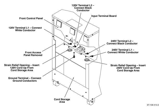
Figure 4-1. Input Terminal Board And Ground Connectors
